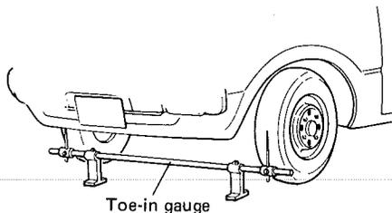
Toe is adjusted by changing tie rod length. Loosen right and left tie rod end lock nuts first and then rotate right and left tie rods by the same amount to align toe-in to specification. In this adjustment, right and left tie rods should become equal in length ("A" in below figure). Before rotating tie rods, apply grease between tie rods and rack boots so that boots won't be twisted.
