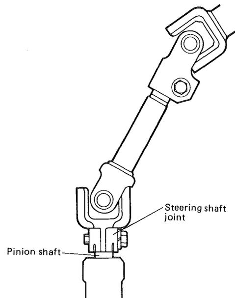
Tighten joint bolt on pinion shaft side, column bolts and then joint bolt ①.
