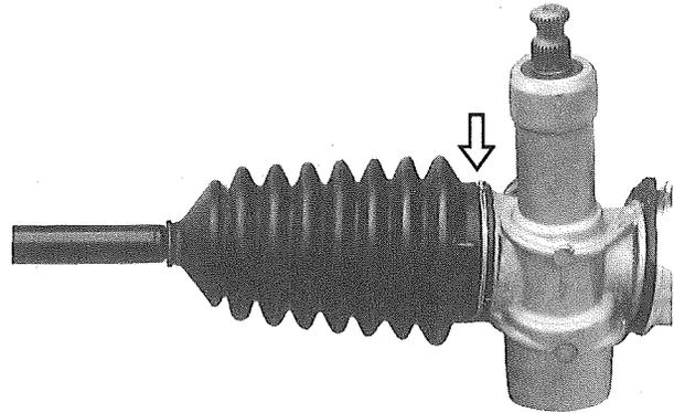
2) Straighten bent lock washer, loosen tie rod ball stud case ① till it is removed from steering rack.
